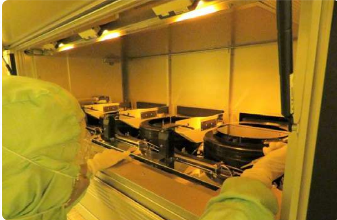
TSMC collaborates with supplier to verify of coating with Next-generation Low Temperature Polyimide formula in lithography process.
